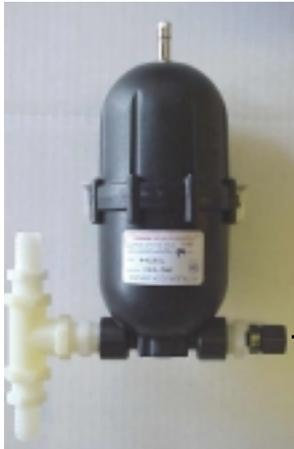
Use accumulator port to connect the pressure gauge. Tubing must be pressure rated to 150 PSI (10 BAR)
