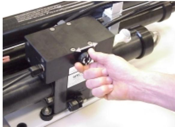
2. Turn on the feed water pump. Check that it is primed by inspecting the brine discharge.
