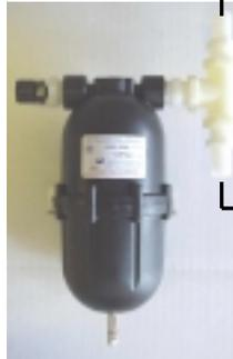
**Spectra Clark Pump**. Mount in a cool location. May be oriented in any position and can be well above waterline. Leave access to the pressure relief valve. Do not mount over electrical equipment. Use supplied spacers and washers for the vibration mounts.
