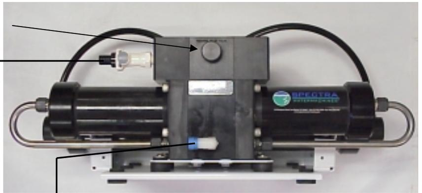
Plastic fittings should have 3-4 wraps of Teflon tape and will thread almost all the way in. Leave the first pipe thread uncoated. Avoid getting dirt or debris in the system during assembly. Avoid tight bends and elbows. Secure piping away from moving objects and protect from chafe.
